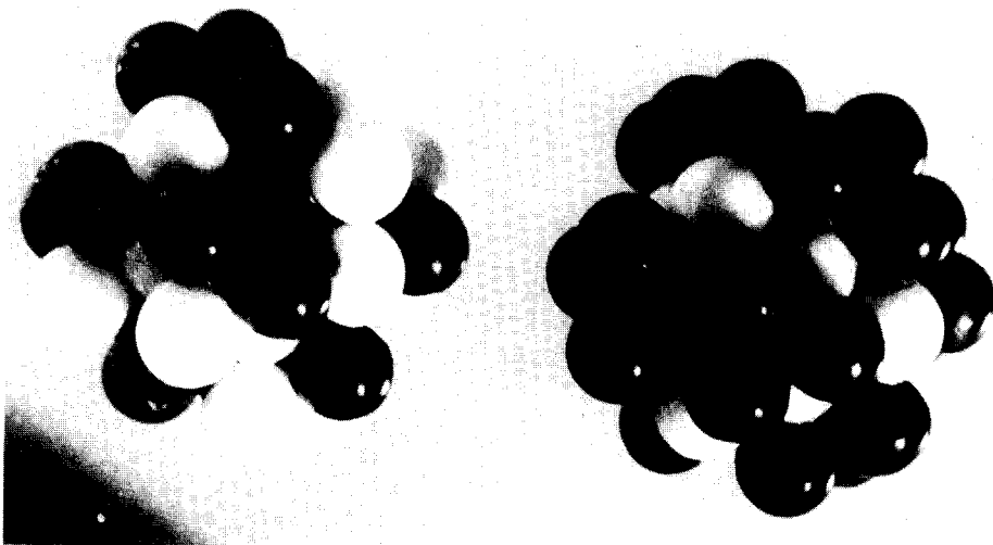
FIG. 2. Photographs of hard sphere models of microcrystals of 43 atoms showing a random atomic arrangement, left, and segregation of one component to the corners and edges, right.
